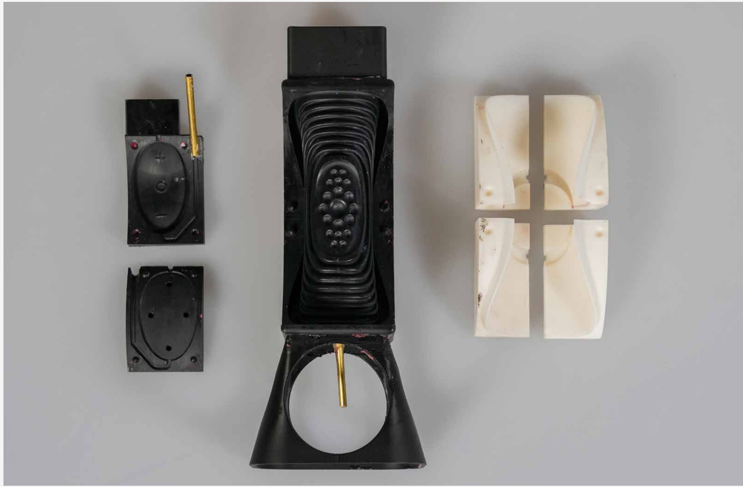
3D-printed mold for casting silicone in a vacuum
